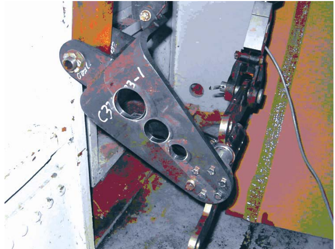
The trailing arm is now thinner with 1 top and 3 side holes.
