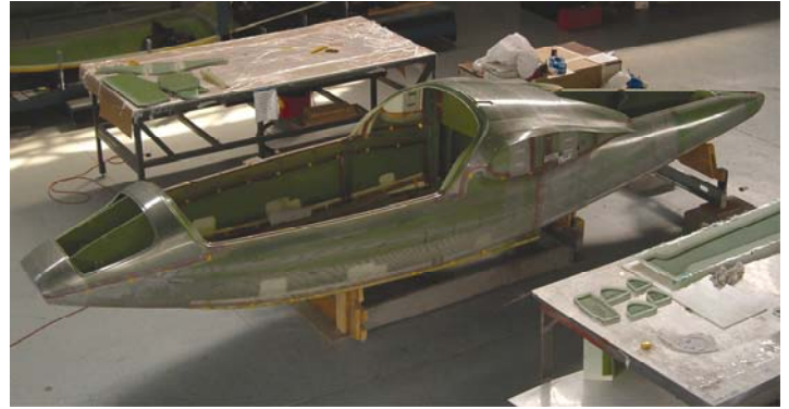
The hull is ready for the vertical tail and scheduled to be tested
