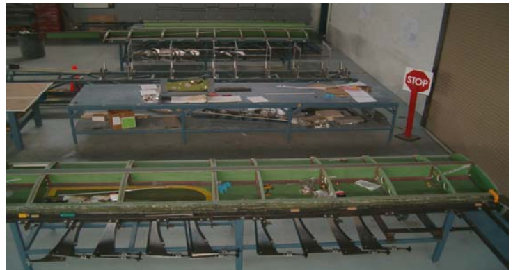
Two wings in the process of production.
