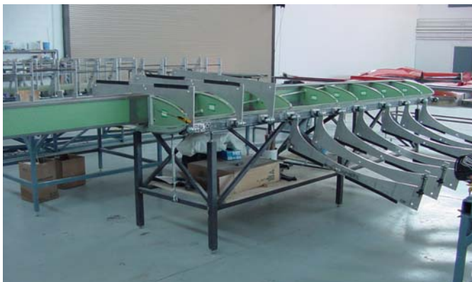
The spar/rib assembly installed in the left & right wing assembly fixture to complete the wing and sponson.
