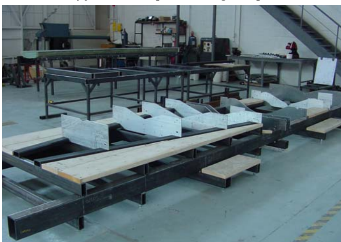
The hull fixture is complete
