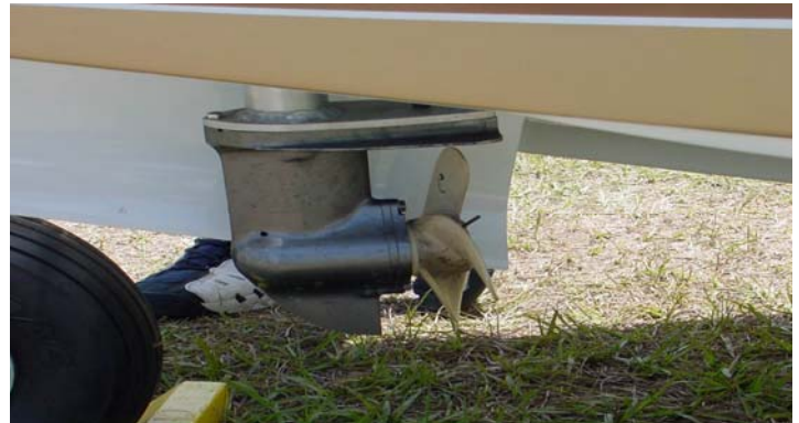
The propeller goes down through the hull
