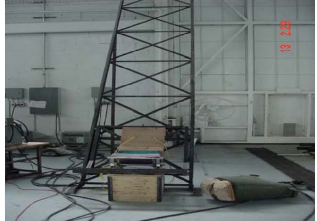
The seat drop test simulates the 19g 60 degree vertical test
