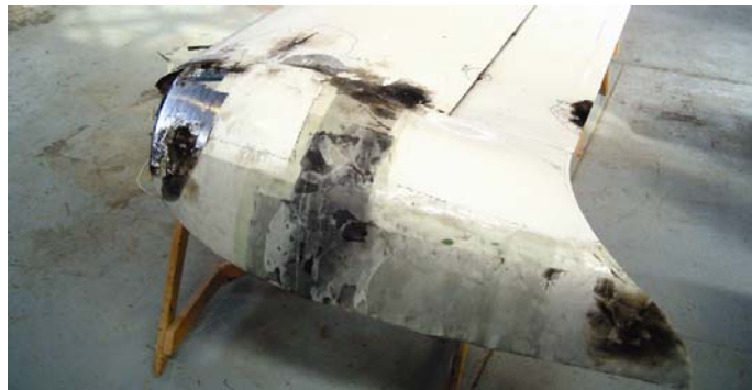
After passing all the wing load and landing gear tests the wing sustained eight lightning strikes
