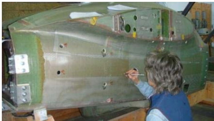
One repair procedure on the right fuselage and over 80 visible open holes in the one wing and mid fuselage.
