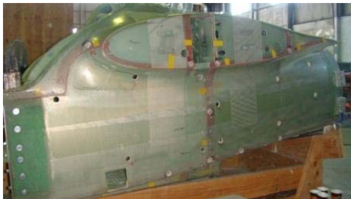
Visible hole damage was added on the left side of the fuselage midsection.
