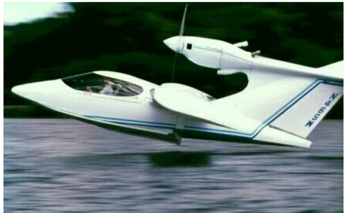
This is the perfect angle for landing on water. The step should touch at the same time as the stern.
