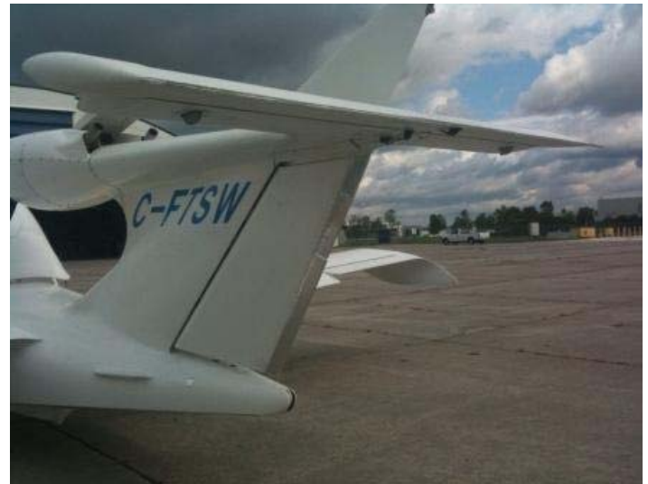
For flight testing, the modifications are covered with speed tape. That's why you see a silvery band on the trailing edge. That won't be on the production Seawind. The production molds will have to be modified.
