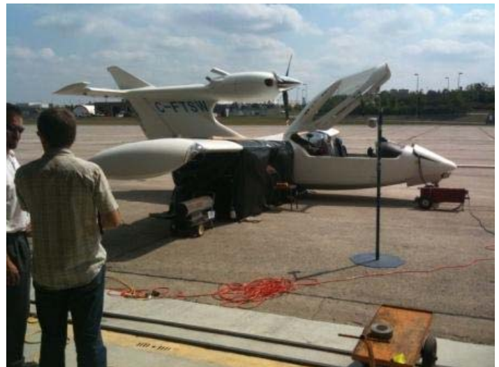
Using a 1,000,000 BTU heater and a black plastic tent we heated the fuel to 111°F.
