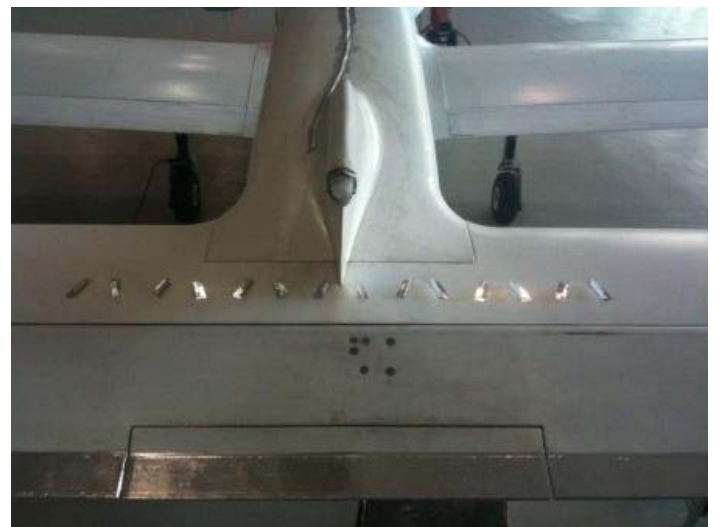
The VGs enhanced the elevator trim tab for rotation.
